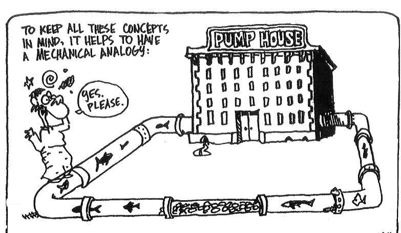
IMAGINE THAT ELECTRIC CURRENT IS LIKE WATER FLOWING THROUGH A PIPE. THEN WE HAVE THESE CORRESPONDENCES:
