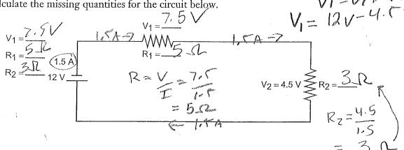
3. Calculate the missing quantities for the circuit below.
